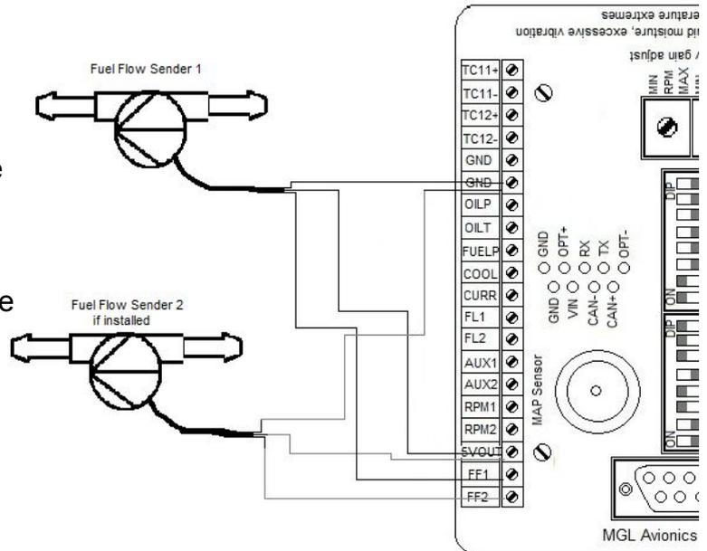
It is also important to work out what fuel flow to expect (generally manufacturers specify fuel usage per hour) in order to select the right jet for the fuel flow sender unit.
