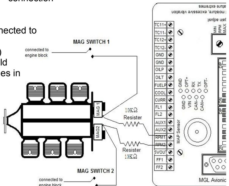
Rev counter pickup for Stratomaster instruments fitted to automotive engines
