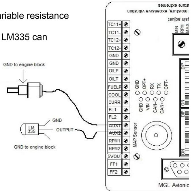
This is a typical Rotax 912/914 CHT sensor connection. With this setup the AUX 1 PU and AUX 2 PU switches will be in the ON position.
