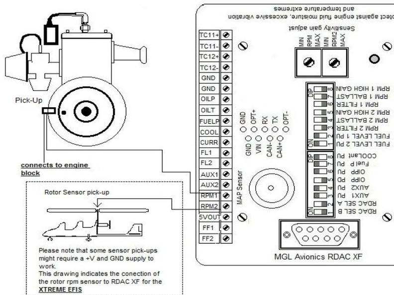
On the EFIS AND IEFIS units the RPM generally works by taking the highest RPM reading for display on the standard screens.
