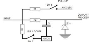
These circuits shows how the various PU switches feeds 5 volt onto the input(sense) line if required. Please check the senders information for type and settings needed. The 2<sup>nd</sup> circuit shows a pull down circuit that has a 100Ω load resistor switched to GND. This intended for use with the Rotax 4-20 mA oil pressure sender. The white wire is connected to the OILP input on the RDAC XF. The OILP PD switch must be in the ON position and the OIL PU switch must be in the OFF position.
